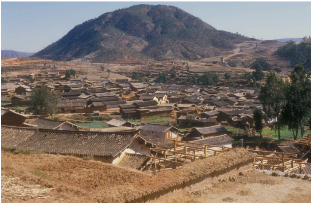
Figure 3-9: A tightly packed village: Yishala in Panzhihua, Sichuan. Mud walls in the foreground, whitewashed on many of the houses. The wooden frame of a house under construction will be filled in with mud walls and a tile roof. The mountain in the background was traditionally forest commons. Photo by the author.
